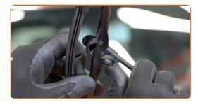
Remove the blade from the wiper arm.
