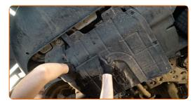
Tighten the fasteners of the oil pan lower cover. Use a drive socket #10. Use a ratchet wrench. Use a Phillips screwdriver.
