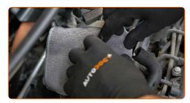
Remove the spark plug wire connectors from the spark plug wells. Use pincers.
