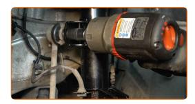
Unscrew the fasteners connecting the stabiliser link to the stabiliser bar. Use a drive socket #15. Use a ratchet wrench.
