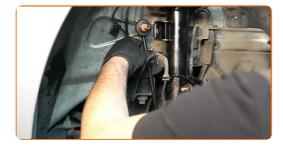
Tighten the fastener connecting the stabilizer link to the shock strut. Use a drive socket #17. Use a torque wrench. Tighten it to 50 Nm torque.
