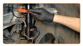
Install a new rod, tighten the fasteners. Use a combination spanner #17. Use a drive socket #17. Use a ratchet wrench.
