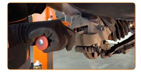
Remove the brake caliper.
