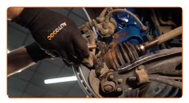
Tighten the brake caliper bracket. Use a drive socket #19. Use a torque wrench. Tighten it to 57 Nm torque.
