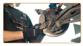
15 Remove the brake disc.
