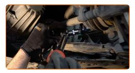
Remove the hydraulic transmission jack.
