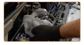
17 Reinstall the air filter housing.
