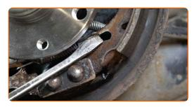
Remove the hold-down pins of the brake shoes. Use round-nose pliers.
