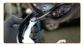
Install the brake shoes on the working brake cylinder on the bracket and on the brake-support plate bracket.
