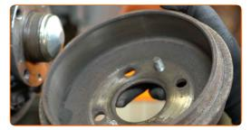
Clean the fasteners of the brake shoes. Use a wire brush. Use WD-40 spray.
