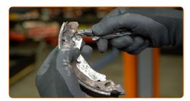
Clean the mounting seats of the brake shoes. Use a wire brush. Use all-purpose cleaning spray.
