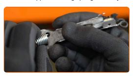
Connect the parking brake cable to the parking brake lever.
