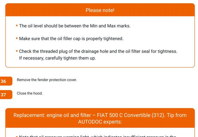
• Note that oil pressure warning light, which indicates insufficient pressure in the lubrication system, may be on for a longer time than usual. After a few seconds, the oil will fill all the channels, and the light will go out.
