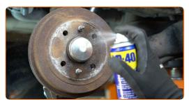
Unscrew the brake drum fastening. Use a drive socket #12. Use a ratchet wrench.
