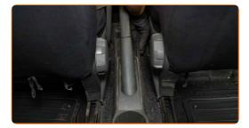
Screw in the front fasteners of the lower centre console. Use a drive socket #10. Use a ratchet wrench.
