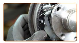
Reinstall the hold-down pins of the brake shoes. Use round-nose pliers.
