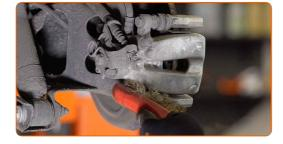
Unscrew the brake caliper fastening. Use a drive socket #13. Use a combination spanner #17. Use a ratchet wrench.
