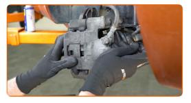
Install the brake caliper cotter pin. Use a pin punch. Use a hammer.
