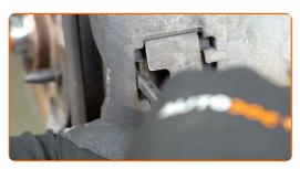
Remove the lock pin retainer clip. Use round-nose pliers.
