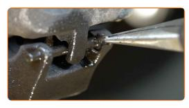
Remove the brake caliper cotter pin. Use a pin punch. Use a hammer.
