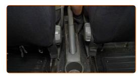
Screw in the front fasteners of the lower centre console. Use a drive socket #10. Use a ratchet wrench.
