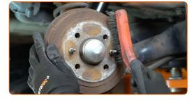
Unscrew the brake drum fastening. Use a drive socket #12. Use a ratchet wrench.
