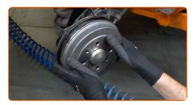
Screw in the brake drum fastener. Use a drive socket #12. Use a ratchet wrench.
