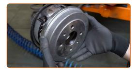
Move the parking brake shoes against the drum. Use a flat screwdriver.
