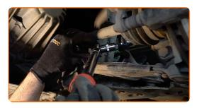
Remove the hydraulic transmission jack.
