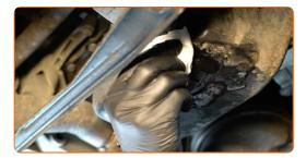
Screw in the new drainage plug and tighten it. Use a drive socket #19. Use a torque wrench. Tighten it to 22 Nm torque.
