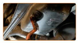
9 Unscrew the drain plug. Use Torx T45. Use a tap wrench.
