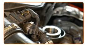
31 Tighten the oil filler cap.
