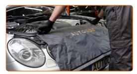
Unscrew the engine cover fastener. Use Torx T25. Use a ratchet wrench.
