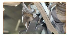
25 Install the brake caliper retaining spring.
