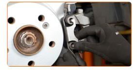
Connect the brake pads wear sensor.
