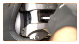
14 Remove the brake caliper.
