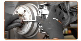
Unscrew the brake caliper fastening. Use HEX No.H7. Use a ratchet wrench.
