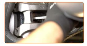
Remove the brake caliper.
