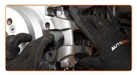
Install the brake caliper retaining spring.
