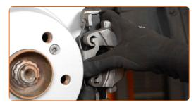
20 Install the wear sensor on the brake pads.
