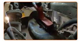
Install the engine mount to its mounting seat.
