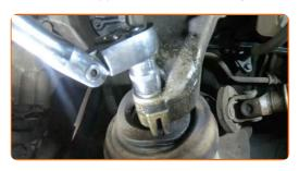
5 Remove the fastening bolt.
