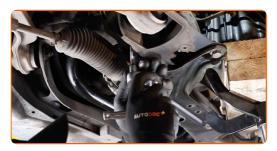
18 Remove the hydraulic transmission jack.
