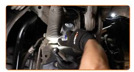
Unscrew the lower fastener of the engine mount. Use a drive socket #16. Use a ratchet wrench.
