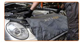
Unscrew the engine cover fastener. Use Torx T25. Use a ratchet wrench.
