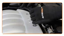
Remove the back section of the engine cover.
