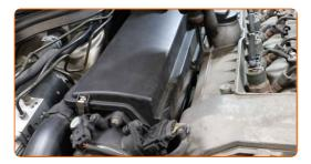
Install the engine cover and secure it.
