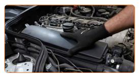
Press the air filter cover clips into place. Use a crowbar.
