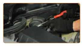
Remove the crankcase ventilation hose. Use a flat screwdriver.
