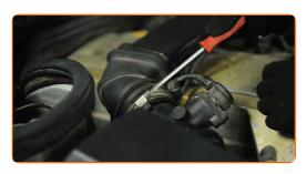
Install the mass air flow sensor.
