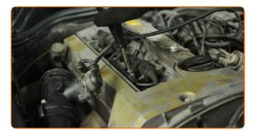
Unplug the connectors from the ignition coils. Use a flat screwdriver.
