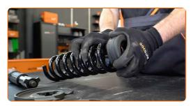
Install a new coil spring on the coil spring compressor.
