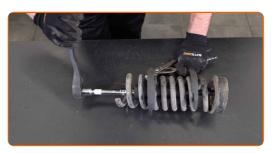
18 Remove the rubber spring spacer.
