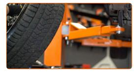
Unscrew the fasteners of the control arm cover. Use a drive socket #10. Use a ratchet wrench.
