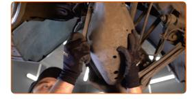
Screw in the fasteners of the control arm cover. Use a drive socket #10. Use a ratchet wrench.
