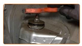
Loosen the upper fastener of the shock absorber. Use a special drive socket to remove the shock absorber # 17. Use a shock absorber socket #DD5.2. Use a ratchet wrench.
