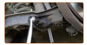
Unscrew the upper fastener of the shock absorber.
