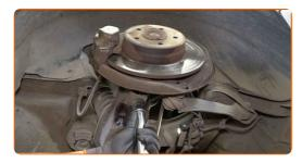
Unscrew the lower fasteners of the shock absorber. Use a combination spanner #16. Use a drive socket #16. Use a ratchet wrench.
