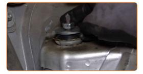
Remove the support from under the rear control arm.
