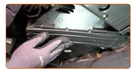
Reinstall the cabin filter cover retainers.
