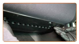
Install the air vent. Use a Phillips screwdriver.
