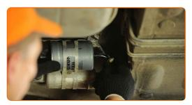
Tighten the fastening clamp of the fuel filter pipe. Use a flat screwdriver.
