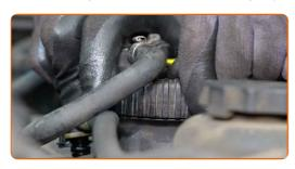
Tighten the fasteners of the fuel filter housing cover. Use a universal puller. Use a torque wrench. Tighten it to 35 Nm torque.
