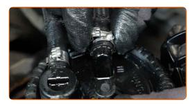
Tighten the fastening clamp of the fuel filter pipe. Use clic-R collar pliers.
