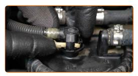
5 Disconnect the pipe from the fuel filter.
