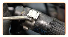
Disconnect the fuel hose from the fuel filter.
