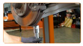
Unscrew the lower fasteners of the shock absorber. Use a combination spanner #17. Use a drive socket #17. Use a ratchet wrench.
