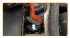
Loosen the upper fastener of the shock absorber. Use a special drive socket to remove the shock absorber # 16. Use a shock absorber socket #DD6. Use a ratchet wrench.
