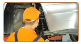
Attach the lower part of the shock absorber. Use a flat screwdriver.
