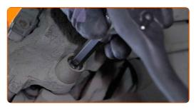
13 Remove the brake caliper.
