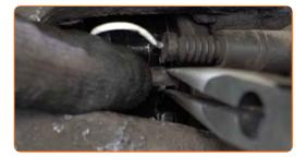
Install the brake pad retaining clip. Use a crowbar.
