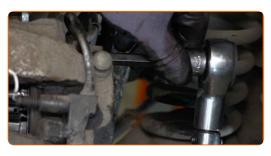
Install the caps on the brake caliper guide pin boots.
