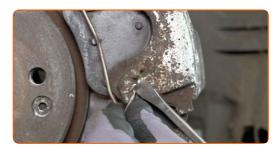
Disconnect the brake pad wear sensor. Use long nose pliers.
