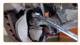
Unscrew the fastener connecting the ball joint to the suspension control arm. Use a drive socket #22. Use a ratchet wrench.
