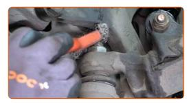
Unscrew the fastener connecting the ball joint to the steering knuckle. Use a combination spanner #22.
