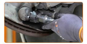
p Disconnect the ball joint from the control arm. Use a ball joint puller.
