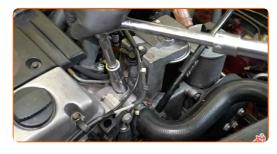
Install a new coolant temperature sensor.
