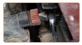
Drain the coolant from the engine.
