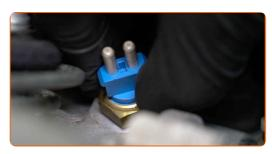
Replacement: temperature sensor and engine thermostat – Mercedes W124.
