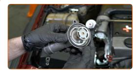
Install the thermostat together with the housing.
