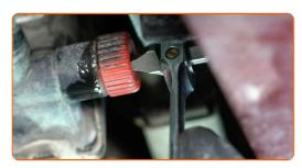
Clean the thermostat housing fasteners. Use a wire brush. Use all-purpose cleaning spray.
