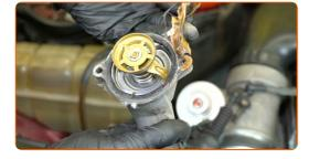
Clean the thermostat housing mounting seat. Use a wire brush. Use all-purpose cleaning spray.
