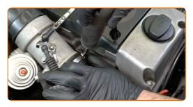
Remove the coolant reservoir cap.
