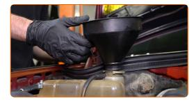
Pour coolant in the coolant reservoir.
