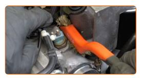
Unscrew the coolant temperature sensor. Use a drive socket #22. Use a ratchet wrench.
