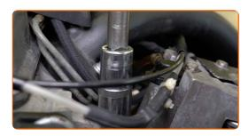
Treat the coolant temperature sensor connector. Use dielectric grease.
