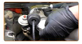
6 Unscrew the coolant reservoir cap.
