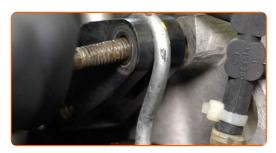
Screw in the fastening bolt of the belt tensioner. Use a combination spanner #16 (2 pieces).
