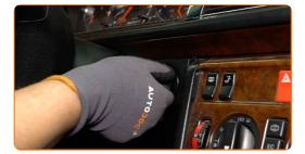
Switch on the air conditioning system. This is necessary in order to make sure that the component operates properly.
