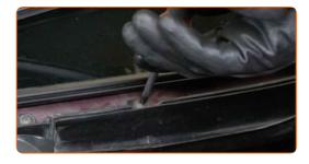
6 Remove the side part of the drain.
