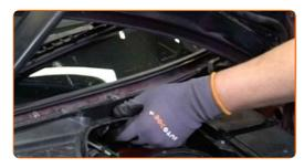
Screw in the fasteners of the drain. Use a Phillips screwdriver.
