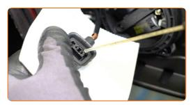
Attach the mirror heater connector.
