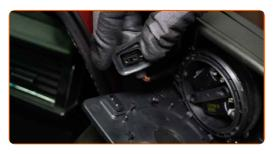
Treat the mirror heater connector. Use dielectric grease.
