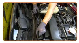
Remove the central element that holds the seal of the windscreen wiper scuttle tray.
