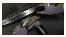
Clean the wiper motor fasteners. Use a wire brush. Use WD-40 spray.
