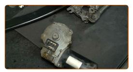
Clean the wiper motor mounting seat. Use a wire brush. Use all-purpose cleaning spray.
