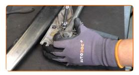
Clean the wiper motor connector. Use dielectric grease.
