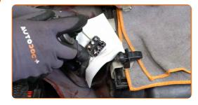
Clean the mounting seat of the windscreen wiper mechanism. Use a wire brush. Use all-purpose cleaning spray.
