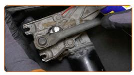
Unscrew the fastener connecting the linkage to the wiper motor shaft. Use a drive socket #13. Use a ratchet wrench.
