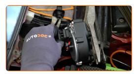
Tighten the windscreen wiper mechanism fasteners. Use a drive socket #10. Use a torque wrench. Tighten it to 13 Nm torque.
