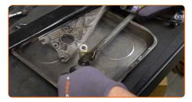
22 Install a new wiper motor.
