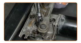
Unscrew the wiper motor fasteners. Use a drive socket #10. Use a ratchet wrench.
