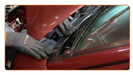
Install the central element that holds the seal of the windscreen wiper scuttle tray.
