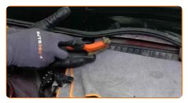
Install the windscreen wiper mechanism.
