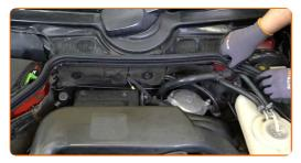
Remove the fender protection cover.
