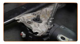
25 Install the wiper linkage on the motor shaft. Use a ruler.
