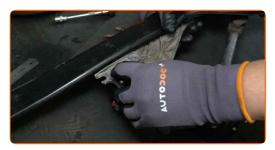
Tighten the wiper motor fasteners. Use a drive socket #10. Use a torque wrench. Tighten it to 13 Nm torque.
