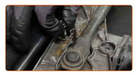
Detach the wiper linkage from the motor shaft.
