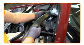
6 Unscrew the fasteners of the drain. Use a Phillips screwdriver.
