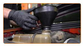
Pour coolant in the coolant reservoir.
