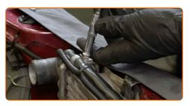
Detach the expansion tank hose from the radiator.
