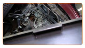
Open the coolant drain tap. Use a flat screwdriver.
