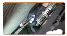
Unscrew the fastener of the lower automatic transmission cooler line. Use a drive socket #10. Use a ratchet wrench.
