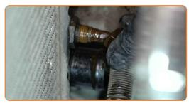
Remove the upper engine radiator clips. Use a clip removal tool.
