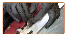
Attach the automatic transmission cooler lines to the radiator.
