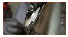
Clean the fastener of the lower automatic transmission cooler line. Use a wire brush. Use WD-40 spray.
