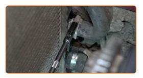
Detach the lower coolant hoses. Use a clip removal tool.
