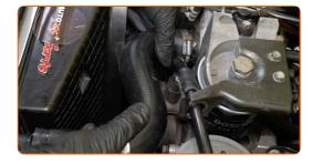
Tighten the clamps of the upper coolant hose. Use a drive socket #7. Use a ratchet wrench.
