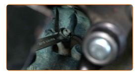
O Drain the coolant from the engine.
