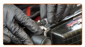
Tighten the clamp of the expansion tank hose. Use a drive socket #7. Use a ratchet wrench.
