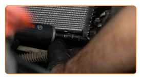
Screw in the fastener of the lower automatic transmission cooler line. Use a drive socket #10. Use a ratchet wrench.
