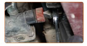
Drain the coolant from the engine.
