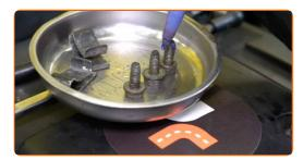
Tighten the fan fasteners. Use a drive socket #10. Use a torque wrench. Tighten it to 10 Nm torque.
