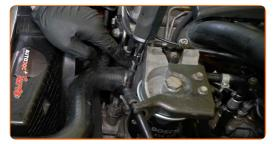
Remove the coolant reservoir cap.
