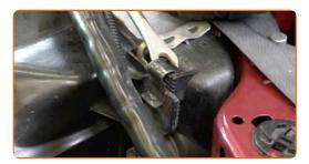
Loosen the clamps of the upper coolant hose. Use a drive socket #7. Use a ratchet wrench.
