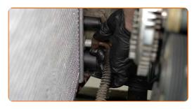
Screw in the fasteners connecting the automatic transmission cooler lines to the radiator. Use a combination spanner #19.
