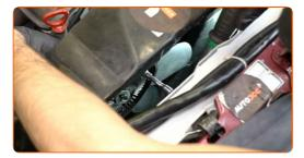
Install the fan shroud clips.
