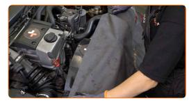
Release the air filter cover clips.
