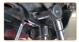
Tighten the fastener connecting the sway bar link to the suspension arm. Use a combination spanner #13. Use a drive socket #13. Use a torque wrench. Tighten it to 40 Nm torque.
