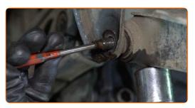
Detach the control arm from the subframe and lower the hydraulic transmission jack. If necessary, use a crowbar.
