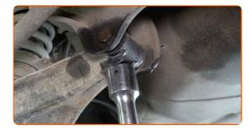
Unscrew the fastener connecting the control arm to the subframe. Use a combination spanner #19. Use a drive socket #19. Use a ratchet wrench.
