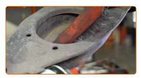
Clean the suspension arm mounting seats. Use a wire brush. Use all-purpose cleaning spray.
