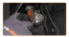
Loosen the upper fastener of the shock absorber. Use a combination spanner #17. Use a shock absorber socket #DD5.2. Use a ratchet wrench.
