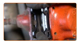
Install the retaining spring of the brake pads.
