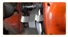
16 Install the brake pad guide pins. Use a pin punch. Use a hammer.
