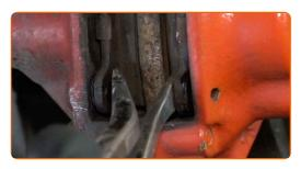
12 Remove the brake pads.
