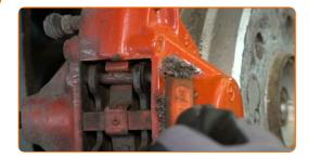
Remove the brake pad guide pins. Use a pin punch. Use a hammer.
