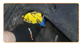
Clean the mounting seat of the suspension strut mount. Use a wire brush. Use all-purpose cleaning spray.
