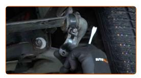
Remove the coil spring together with the coil spring compressor.
