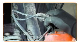
Unscrew the lower fasteners on the shock absorber. Use a drive socket #19. Use a ratchet wrench.
