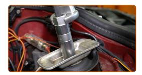
Tighten the fasteners of the upper strut mount. Use a drive socket #13. Use a torque wrench. Tighten it to 20 Nm torque.
