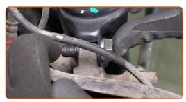
Tighten the lower fasteners on the shock absorbers. Use a drive socket #19. Use a torque wrench. Tighten it to 110 Nm torque.
