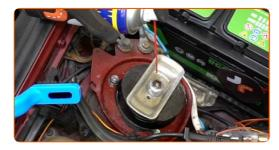
Loosen the fasteners of the upper strut mount. Use a drive socket #13. Use a ratchet wrench.
