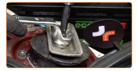
Unscrew the fasteners of the upper strut mount. Use a drive socket #13. Use a ratchet wrench.
