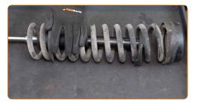
Put the coil spring compressor on the new spring.
