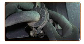
Tighten the fasteners on the anti-roll bar bush brackets. Use a combination spanner #13. Use a drive socket #13. Use a torque wrench. Tighten it to 20 Nm torque.
