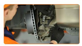
Unscrew the rod end fastening. Use a drive socket #16. Use a ratchet wrench.
