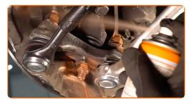
Tighten the rod end fastening. Use a drive socket #16. Use a torque wrench. Tighten it to 40 nm torque.
