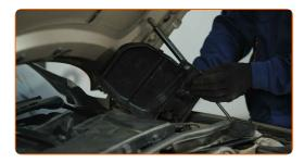
Unscrew the fasteners of the cowl grille. Use a drive socket #8. Use a ratchet wrench.
