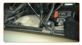
Attach the electrical wiring to the upper part of the microfilter housing.
