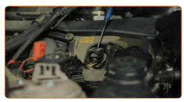
Take out the ignition coils from the spark plug wells. Use a flat screwdriver.
