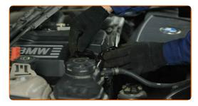
Tighten the oil filler cap.
