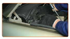
Tighten the fasteners of the cowl grille. Use a drive socket #8. Use a torque wrench. Tighten it to 11 nm torque.
