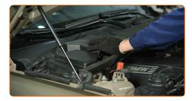
Screw in the fasteners of the cabin filter housing cover. Use a drive socket #8. Use a ratchet wrench.
