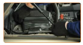
Remove the wiper cowl grille located on the left side. Use a flat screwdriver.
