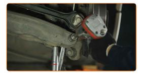
Treat the rear knuckle fasteners. Use copper grease.
