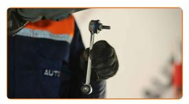
install the rod fastening to the stabilizer and tighten it. Use a drive socket #13. Use a torque wrench. Tighten it to 21 Nm torque.
