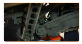
Tighten the fastener connecting the stabilizer link to the stabilizer bar. Use a combination spanner #17 (2 pieces). Use a torque wrench. Tighten it to 58 Nm torque.
