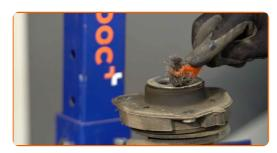
Remove the strut piston rod nut. Use a drive socket #21. Use a ratchet wrench.
