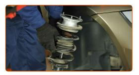
Screw the top fastening of the shock strut mount.
