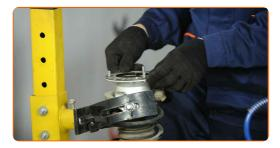
Remove the assembled shock strut.
