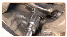
Tighten the front fastener connecting the control arm to the subframe. Use a combination spanner #18. Use a torque wrench. Tighten it to 68 Nm torque.+90°
