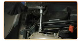
Remove the fender protection cover.
