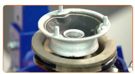
Tighten the shock strut piston rod nut. Use a drive socket #21. Use a torque wrench. Tighten it to 64 Nm torque.
