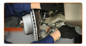
Disconnect the tie rod end from the steering knuckle.
