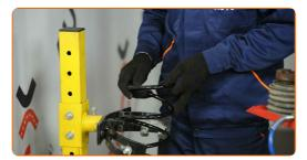
Install the boot and a bump stop onto the shock absorber.
