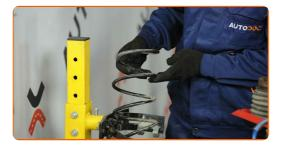
Install the spring on the shock absorber.
