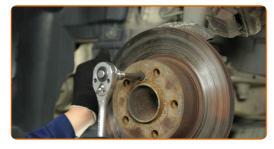
Remove the brake disc.
