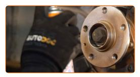
22 Install the brake disc.
