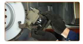
Install the brake caliper and fix it. Use HEX No.H7. Use a torque wrench. Tighten it to 30 Nm torque.
