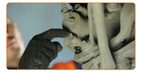
Install the brake caliper retaining spring. Use a flat screwdriver.
