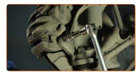
Remove the brake caliper.
