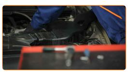
Undo the fastening screws of the air filter cover. Use Torx T25. Use a ratchet wrench.
