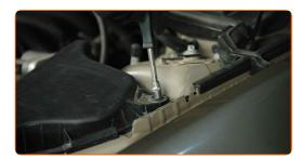
Unscrew the clamp that fastens the air filter hose to the throttle body. Use a flat screwdriver.
