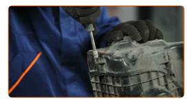
Reinstall the air filter housing.
