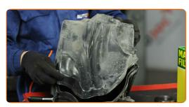
Screw in the fastening screws of the air filter cover. Use Torx T25. Use a ratchet wrench.
