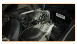
Fasten the clamp on the air intake hose. Use a flat screwdriver.
