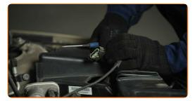
Remove the fender protection cover.
