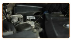
Screw the filter housing fastening bolts. Use a drive socket #10. Use a ratchet wrench.
