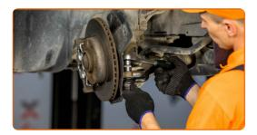
Tighten the tie rod end locknut. Use a combination spanner #24. Use a torque wrench. Tighten it to 55 nm torque.
